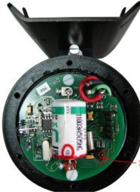
Insert new battery (watch polarity!) and screw down the terminal screws. Correct battery position is shown on the image.
