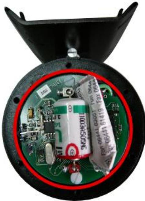
If you have spare parts, replace the o-ring in groove with a new one (52 x 2.5 mm).
