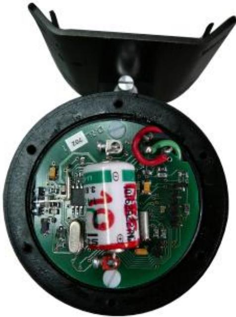
Loosen the battery terminal plug screws and remove the old battery.
