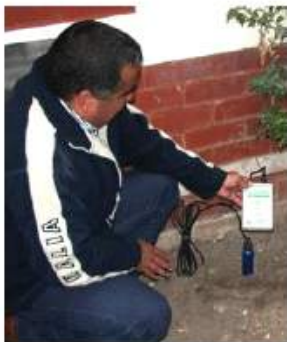
The MPKit can measure to any depth down an augered hole.
