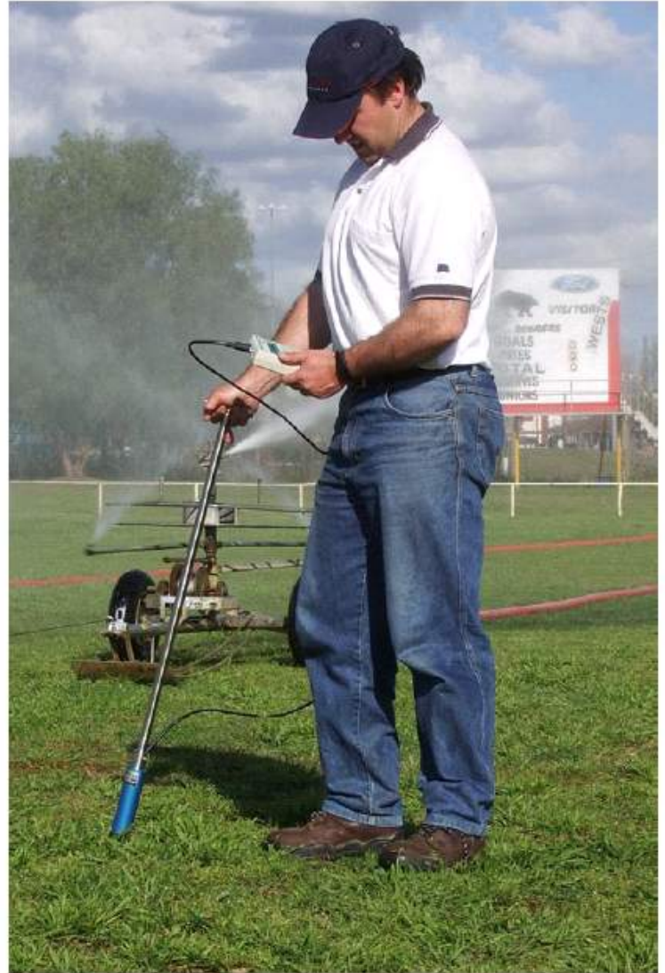
The MPKit measuring surface volumetric moisture content.
