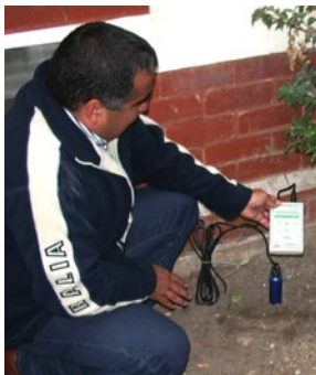
The MPKit can measure to any depth down an augered hole.
