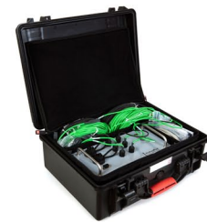
TRSYS01 High accuracy thermal resistance measurement system with 2 measurement locations
