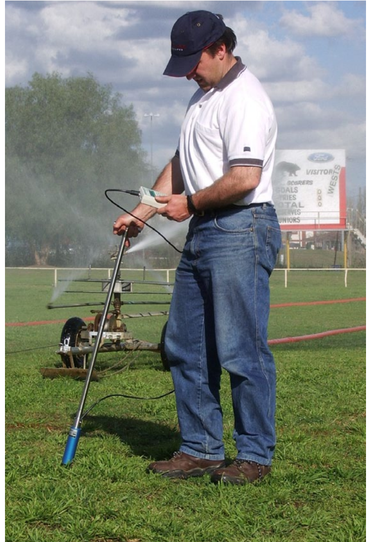
The MPKit measuring surface volumetric moisture content
