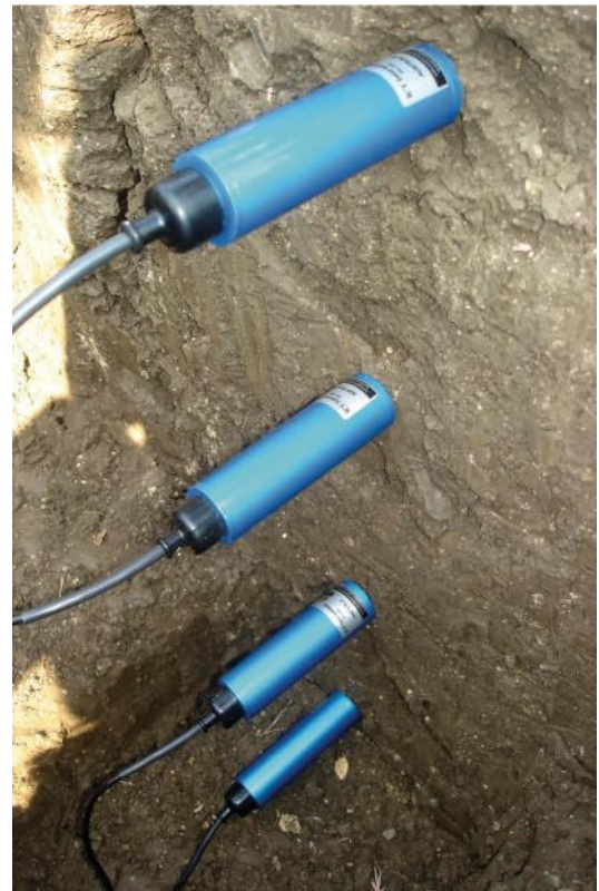
MP406's installed in a soil profile
