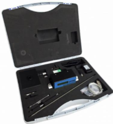
The RIMIK CP300 Cone Penetrometer is used to measure soil density and hardness where a research level study of the data is required. It has been designed for use by those who require data to conduct transverse analysis and low level spatial variation of known locations. It measures and records cone index values based on the load required to force a cone through the soil. The instrument will record profile data to a maximum depth of 750mm.
