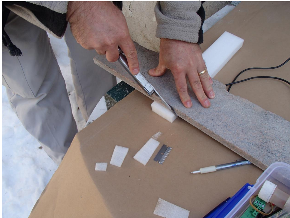
Preparing spacers for HFD installation using polyethylene foam.
