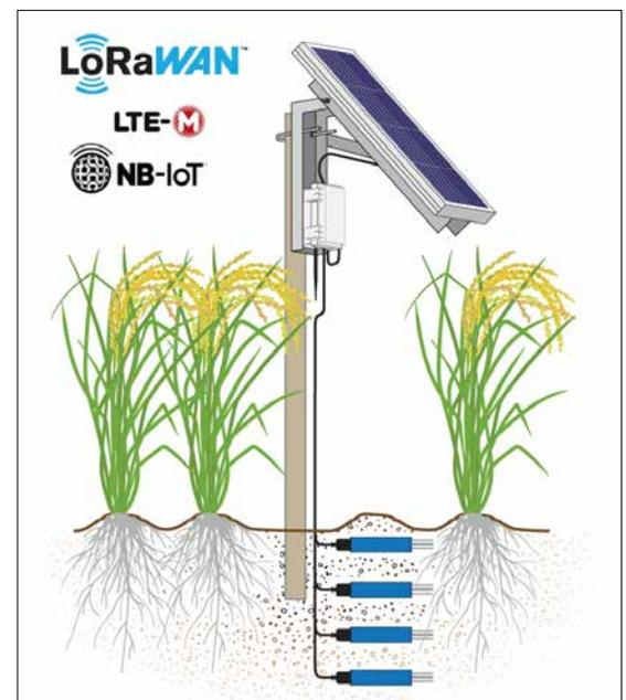
*The SNiP-MP4 is a 'Sensor Node Integrated Package' for LoRa, LoRaWAN, or CAT-M1 communication of real-time accurate soil moisture measurements for continuous soil monitoring. The base SNiP-MP4 integrates 1x MFR-NODE and 1x MP406 soil moisture probe to a site's unique network, communication and power requirements. An added 3x MP406 soil moisture probes can monitor soil moisture at multiple depths.*
