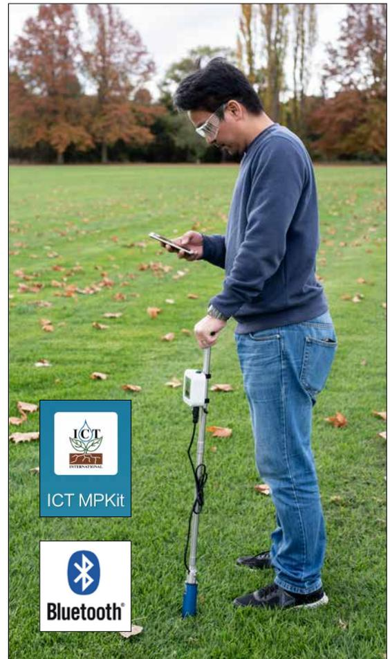
*The MPKit Measuring Surface Volumetric Moisture Content for Managing Turf Grass*
